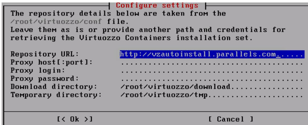
In this window, you can view and, if necessary, configure the following parameters:
