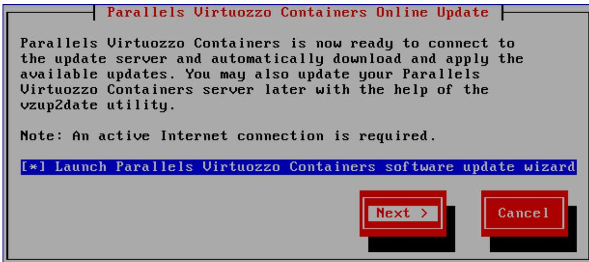
You are highly recommended to check for available updates right during the Parallels Virtuozzo Containers installation. In this case, you will have the latest Parallels Virtuozzo Containers core, utilities, and templates installed once the Parallels Virtuozzo Containers 4.7 installation is complete. To do this:
