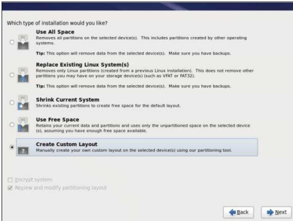
In this window, select the **Create custom layout** radio button as shown in the picture above, and click **Next**. Create the following partitions on the server:
