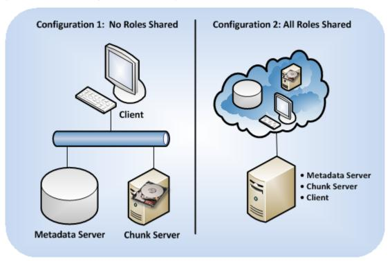
For a Virtuozzo Storage cluster to function, it must have at least one MDS server, one chunk server, and one client. The minimum configuration has two main limitations:
