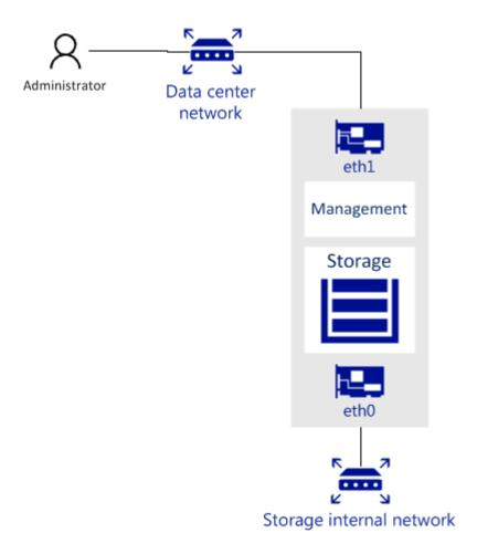
• A node that runs one or more storage access point services must have a network interface for the internal network traffic and a network interface for the public network traffic.
