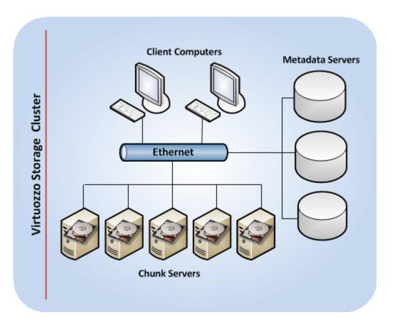
The basic component of Virtuozzo Storage is a cluster. The cluster is a group of physical computers connected to the same Ethernet network and performing the following roles:
