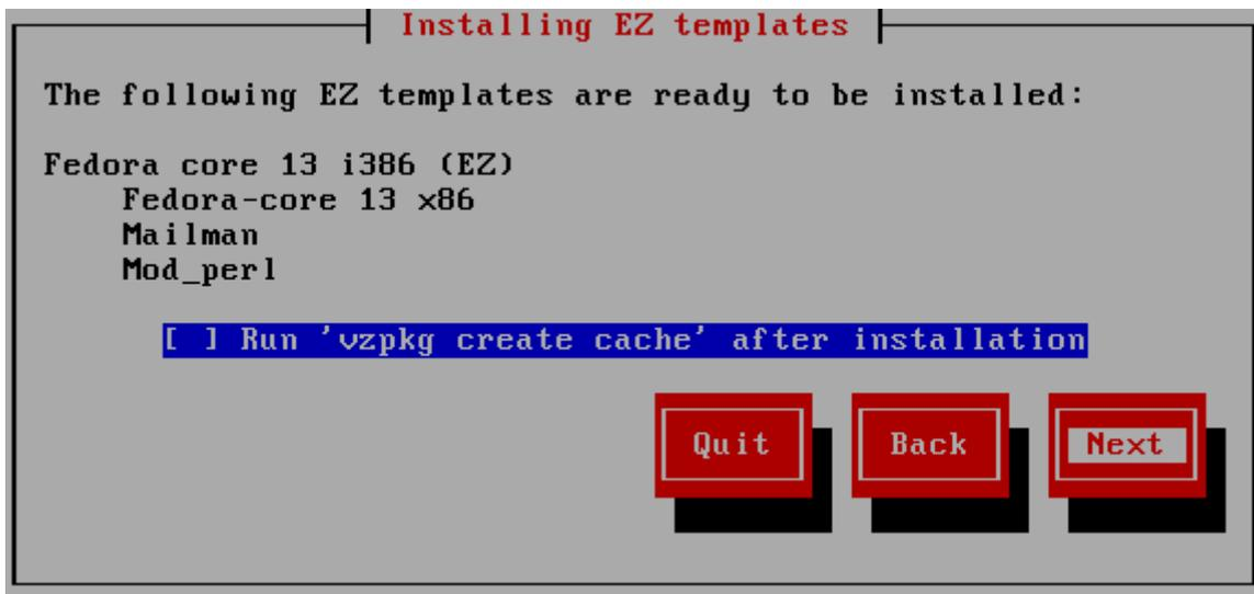
In this window, you can view the templates ready to be installed on your Node. If you are installing a new OS EZ template, you can select the **Run 'vzpkg cache' after installation** check box to cache the OS EZ template right after its installation on the Node. Clicking **Next** starts installing the EZ templates on the Hardware Node.
