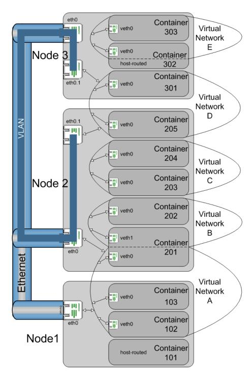
The scheme above illustrates three Virtuozzo physical servers each having a single Ethernet adapter (eth0). The Ethernet adapters are physically united into a single network. On the Ethernet adapters of Nodes 2 and 3, a VLAN is set up.
