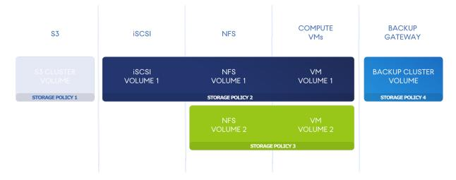
Redundancy means that the data is stored across different storage nodes and stays highly available even if some nodes fail. If a storage node is inaccessible, the data copies on it are replaced by new ones that are distributed among healthy storage nodes. When the storage node goes up after the downtime, out-of-date data on it is updated.
