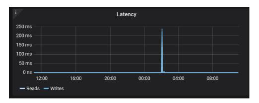
You can also monitor the latency of a particular disk on the **Hardware node details** dashboard:
