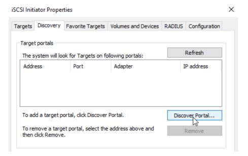
d. In the **Discover Target Portal** window, enter the target IP address and click **OK**. Repeat this step for each target from the target group.
