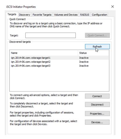
f. Click **Connect** for each target to connect it to the initiator. In the **Connect To Target** window, select the **Enable multi-path** checkbox and click **OK**.
