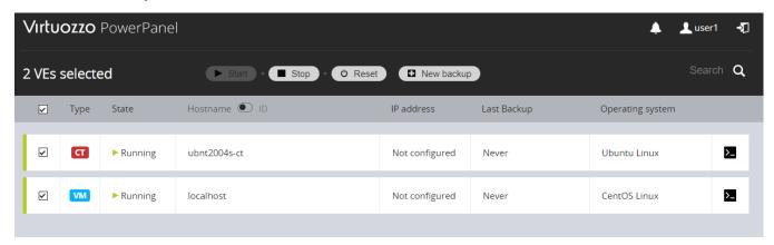
To start, stop, or reset a single VE, you can also click the VE area to expand it, then click the respective task button—**Start**, **Stop**, or **Reset**—in the VE area.
