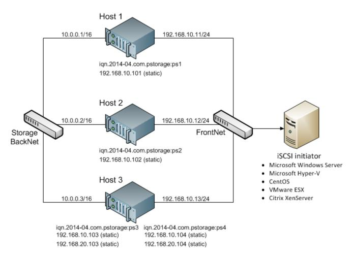
In this example are three Virtuozzo Hardware Nodes working in a Virtuozzo Storage cluster. Two Nodes host one iSCSI target each while the third hosts two iSCSI targets. Each Node has a static or dynamic IP address assigned from the Storage BackNet (created along with the Virtuozzo Storage cluster) and the FrontNet. Each iSCSI target has a static IP address assigned from the FrontNet.
